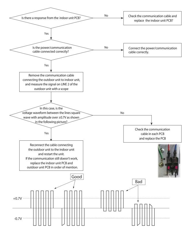
cf.) If there is no oscillo scope, it can be replaced multimeter instead of osillo scope.
