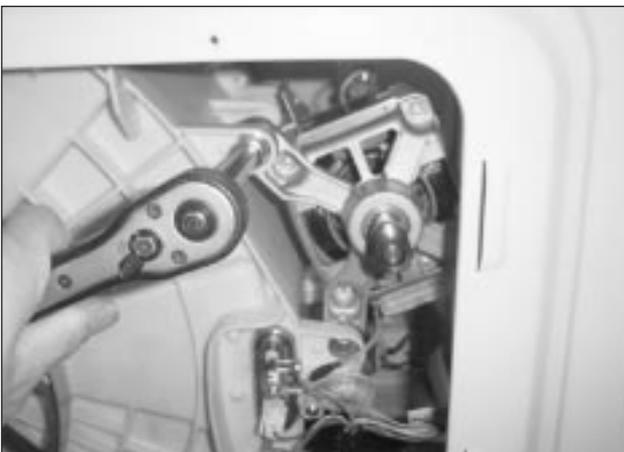
4) Remove the motor from the tub.
