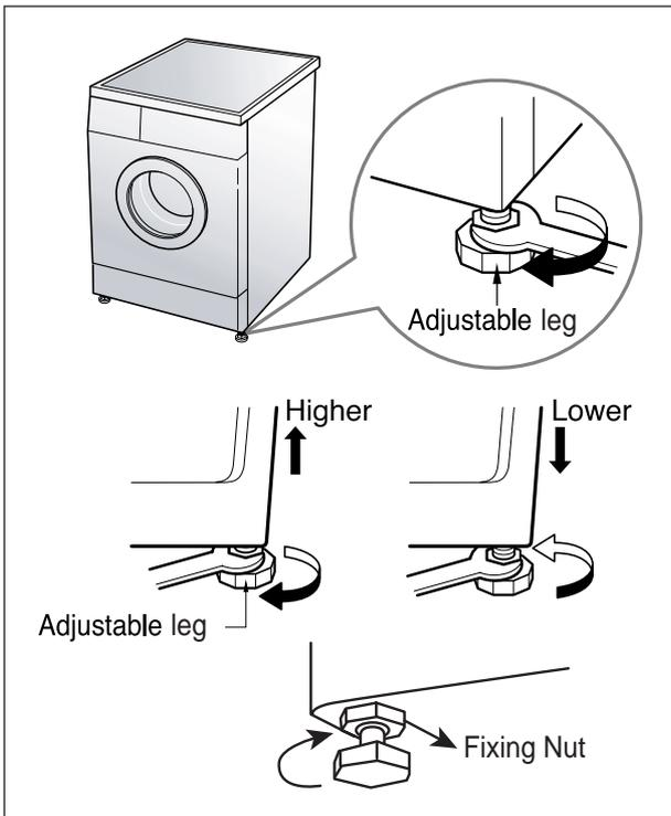
2. If the floor is uneven, adjust the adjustable leg as the following.
