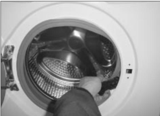
4) Remove two screws, and push the door lock switch to the right direction.
