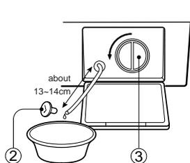
3. Remove any foreign material from the pump filter(③). After cleaning, turn the pump filter clockwise and insert the cap hose(②) to the original place. Close the lower cover.
