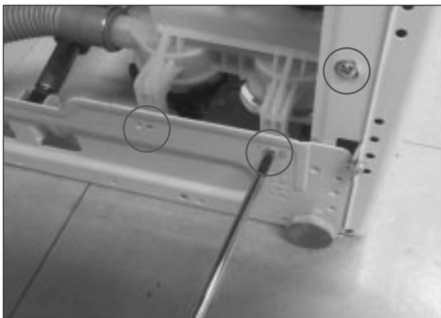
4) Remove the drain hose and the hose water supply.
