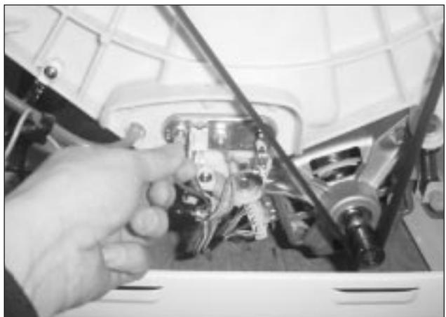
3) Remove the nut by using a box wrench, and remove the earth terminal.
