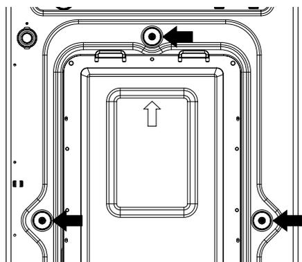
2. Unscrew the 3 bolts with the spanner supplied, and take out the 3 bolts with the rubber bungs. Keep the 3 bolts and the spanner for future use.
