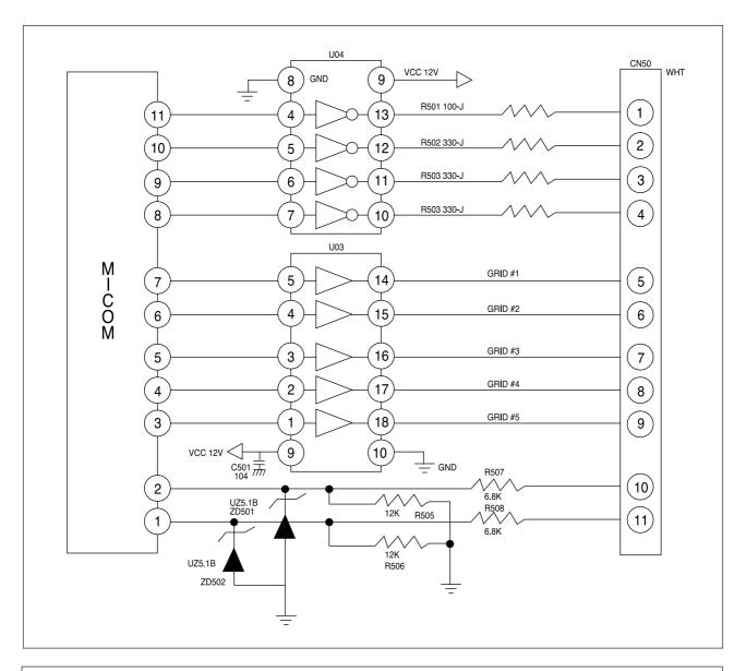
♦from MICOM #3-#7 GHID signal is generated for 10 sec with the period of 2 sec HIGH signal and for the lighting the corresponding LED, the CONTROL terminal of MICOM PIN #8-#11 output the output signal which is coincident with GRID signal. Meanwhile by pushing the KEY which is connected by respective GRID, corresponding signal is inputted to MICOM.
