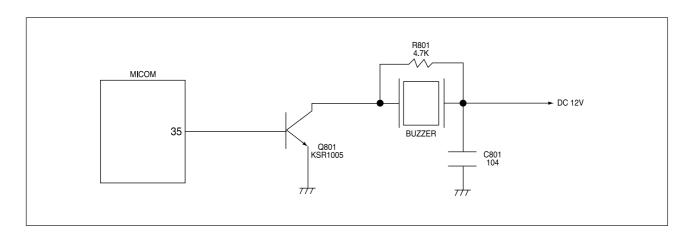
◆ TRANSISTOR begins to operate by CLOCK which was generated at MICOM and BUZZER sound is generated by impression of 12V to the BUZZER.
