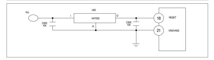
◆ Division of RESET circuit makes it possible that programed function of system is set to be initial state by initializing various parts such as RAM in MICOM when power is impressed or instantaneous electricity failure is occurred. RESET voltage at the impressed moment of power is maintained as "LOW" state for a few seconds and "High" under normal working condition.
