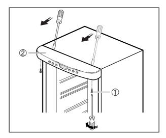
• Repair or change electric parts of top table.
