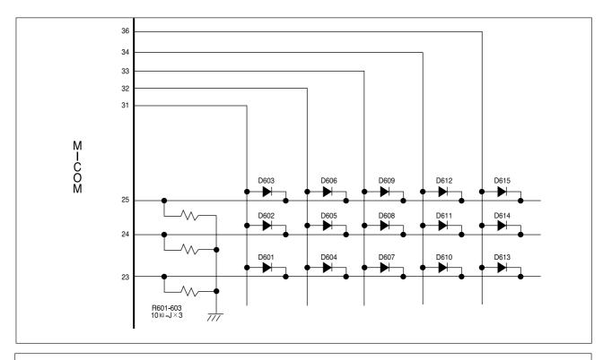
♦ The output such as GRID wave form which is only generated at the initial POWER ON is accepted as input through SWITCHING DIODE and discriminate OPTION by matrix method. #23, #24, and #25 PORT of MICOM PORT generate the same output with GRID wave form only at initial POWER ON.
