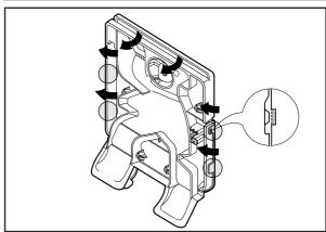
■ Assembly of the cooling cycle unit in the freezer
