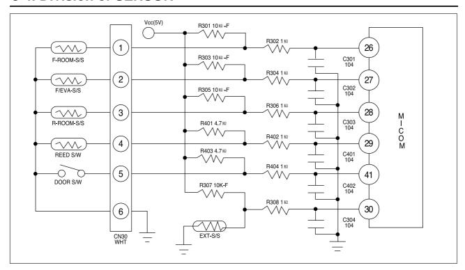
♦ SENSOR and F-rated resistance are connected to the GROUND and DC 5V, respectively. The resistance value which is changed by the temperature is converted to the voltage, and then respective temperature is discriminated by input voltage to A/D PORT of MICOM
